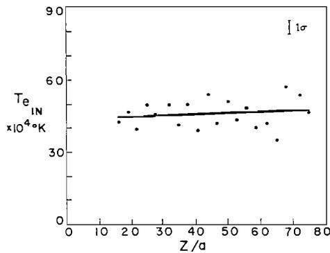
Fig. 3. A plot of the plasma electron temperature  $T_{e,IN}$  on the model centerline downstream from a conducting model with the model in the plasma beam. The least squares line calculated from the data points ( $T_{e,IN} = 0.1(z/a) + 4.2$ ) and the one-sigma bar are also plotted. The vertical and horizontal axes are the same as in Figure 2. The slight increase in value of the least squares line with increasing  $z/a$  is not statistically significant (see text).
