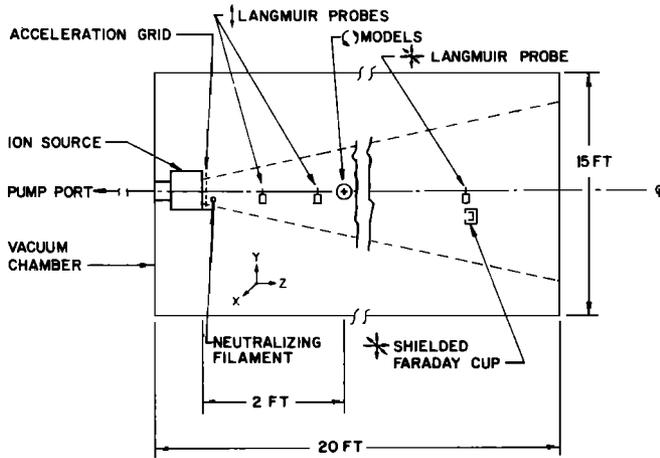
Fig. 1. Schematic representations of the Astrophysical Plasma Laboratory plasma chamber showing the relative locations of the high-energy plasma source, the model, and the various detectors.
