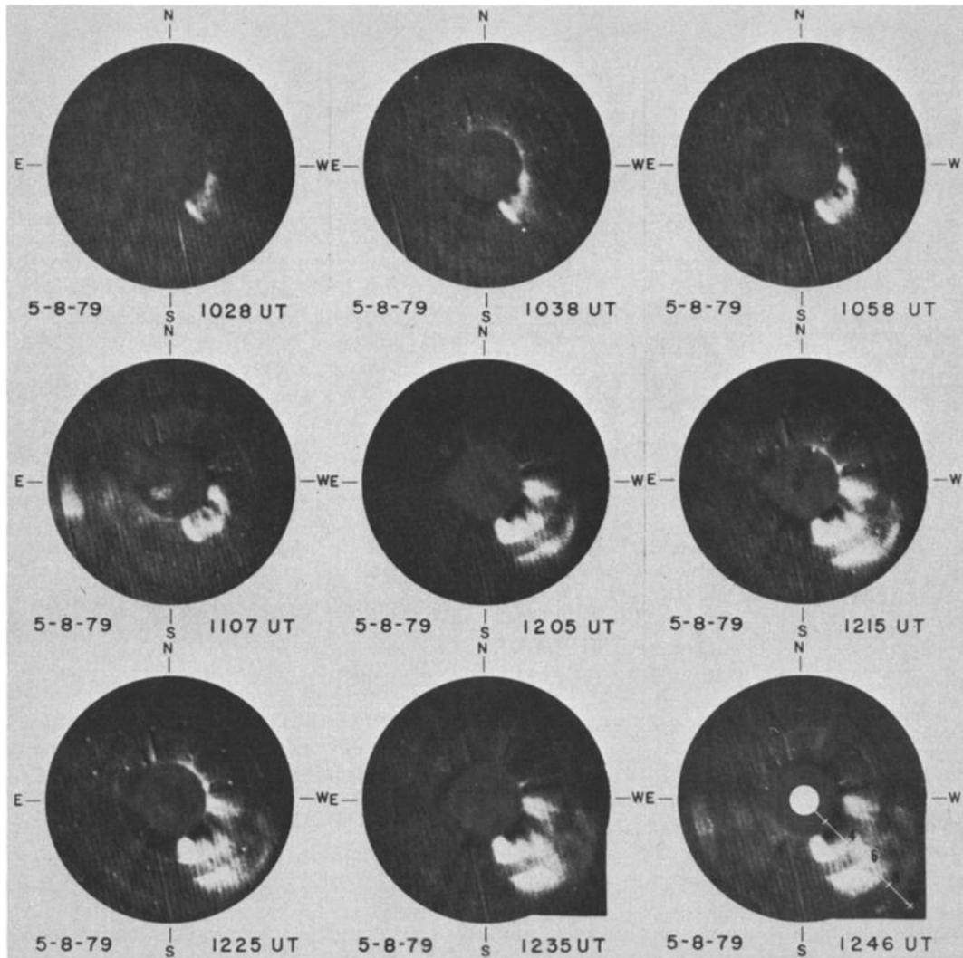
Fig. 4. P78-1 coronal transient (observed by NRL Solwind coronagraph) of May 8, 1979 [from Michels *et al.*, 1980]. The annular ring at  $\sim 5 R_S$  (see the scale at 1246 UT) is caused by a polarizing filter, as noted in the text, and should also be considered as equally bright as the lower and higher radial positions.
