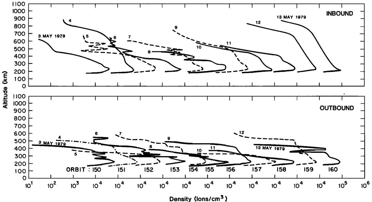
Fig. 9. Sequence of O<sup>+</sup> density profiles in the dayside ionosphere during orbits 150-160 (inbound and outbound) on May 3-13, 1981, respectively, from PVO's ion mass spectrometer (OIMS). Some of the profiles are drawn either with dashes or dash-dots only for convenience in guiding the reader's eye.
