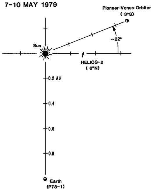
Fig. 1. Schematic sketch (ecliptic plane projection) of the relative positions of the earth (P78-1), Helios 2, and Venus (PVO) during the period May 7-10, 1979. [Note: The 3°S latitudinal figure shown for PVO should read ~0°.]
