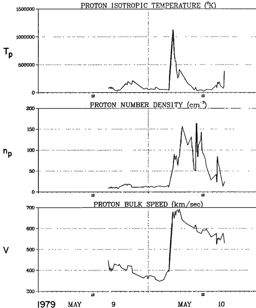
Fig. 7. Solar wind velocity, density, and temperature from PVO's plasma analyzer on May 9–10, 1979.
