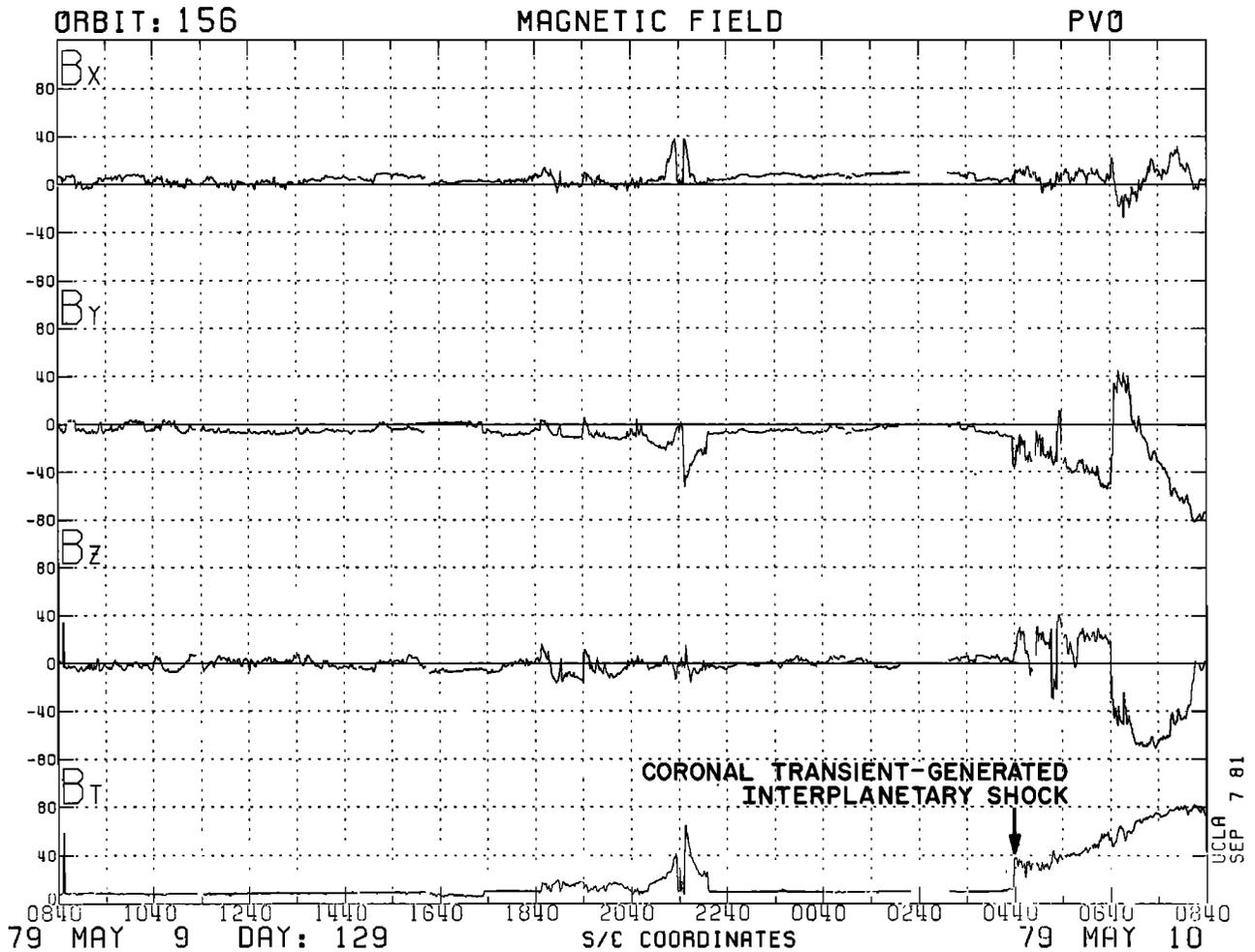
Fig. 6. Solar wind magnetometer data from PVO's magnetometer (courtesy of C. T. Russell and J. G. Luhman of UCLA) on May 9-10, 1979. The perturbation between ~2100-2200 UT is caused by Venus.
